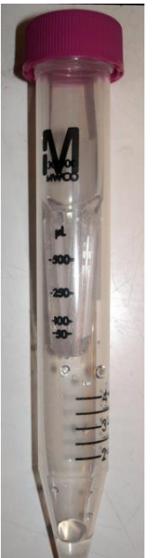
Centrifugation 40 min 3 500 tr/min
